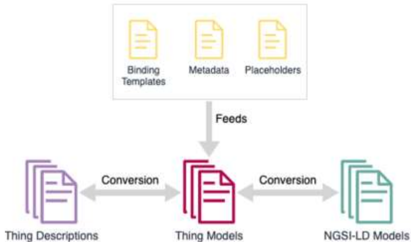
Figure 4-25: Conceptual overview of the semantic mapping between TDs and NGSI-LD models
